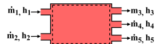
Fig. 4.10: Control volume representation showing multiple inlets and outlets having invariable thermodynamic states with time.
